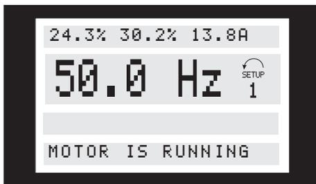
In this state, data values for four operating values are shown at the same time, giving the related unit, cf. table. In the example, Reference, Torque, Current and Frequency are selected as variables in the first and second line.
