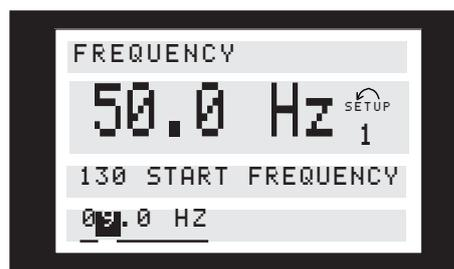
Then the chosen digit is changed infinitely variably by means of the [+/-] keys:
