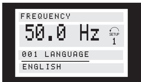
The 3rd line of the display shows the parameter number and name, while the status/value of the selected parameter is shown in line 4.
