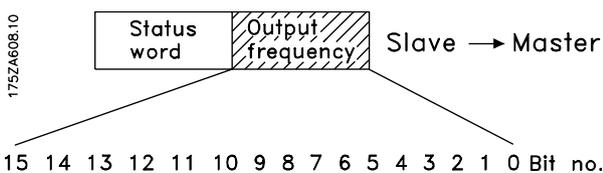
The value of the actual output frequency of the frequency converter is transmitted in the form of a 16-bit word. The value is transmitted as a whole number (0-32767). 16384 (4000 Hex) corresponds to 100%. (Negative figures are formed by means of 2's complement).
