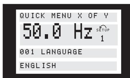
At the bottom of the display, the parameter number and name are given together with the status/value of the first parameter under Quick Setup. The first time the [Quick Menu] key is pressed after the unit has been switched on, the read-outs will always start at pos. 1 - see table below.
