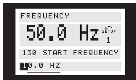
The chosen digit is indicated by the digit flashing. The bottom display line shows the data value that will be entered (saved) when signing off with [OK].
