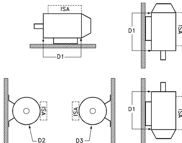
D1: Drain holes opposite inverter side, both drive end and non drive end.
