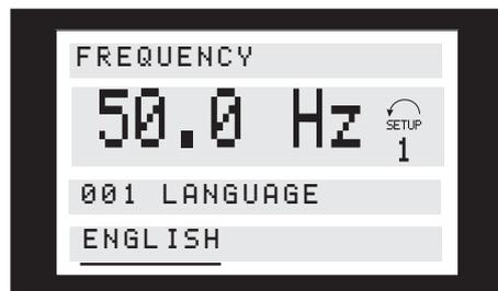
The bottom display line shows the text value that will be entered (saved) when acknowledgement is given [OK].
