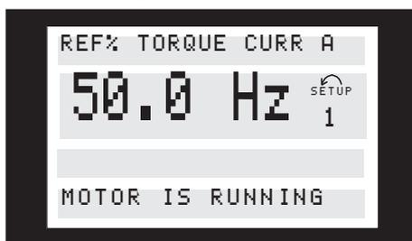
This is where parameter names and units for operating variables in the first line are given - operating variable 2 remains unchanged.
