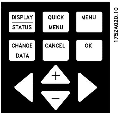
Keys for local control are found under the indicator LEDs.
