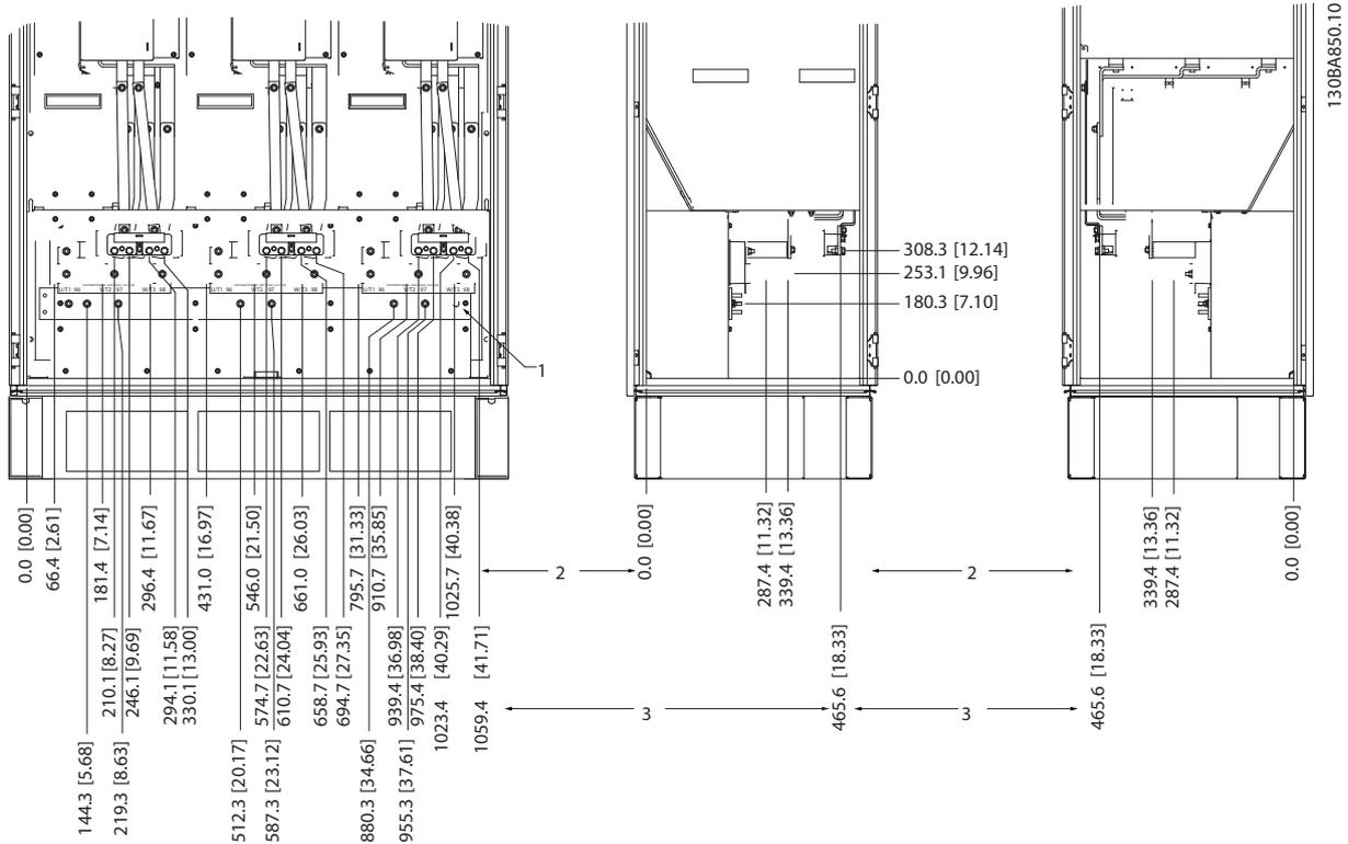
Illustration 5.85 Terminal Locations - Inverter Cabinet - F2 and F4 (Front, Left and Right Side View). The Gland Plate is 42 mm below .0 level.
