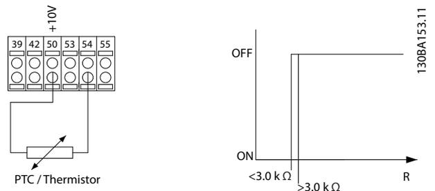
Illustration 2.30 Analog Input 10 V Power Supply
