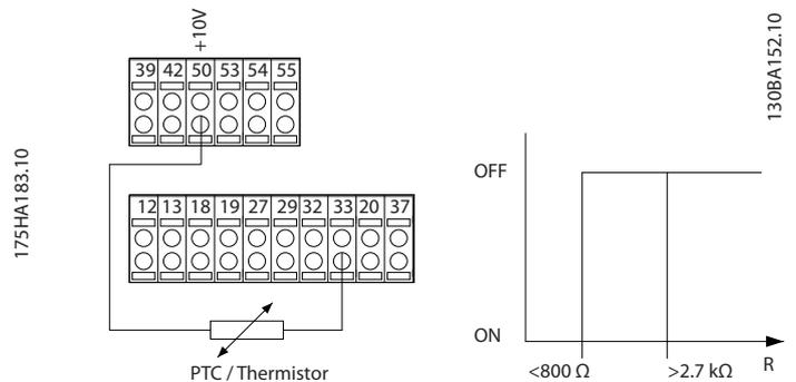
Illustration 2.29 Digital Input and 10 V Power Supply
