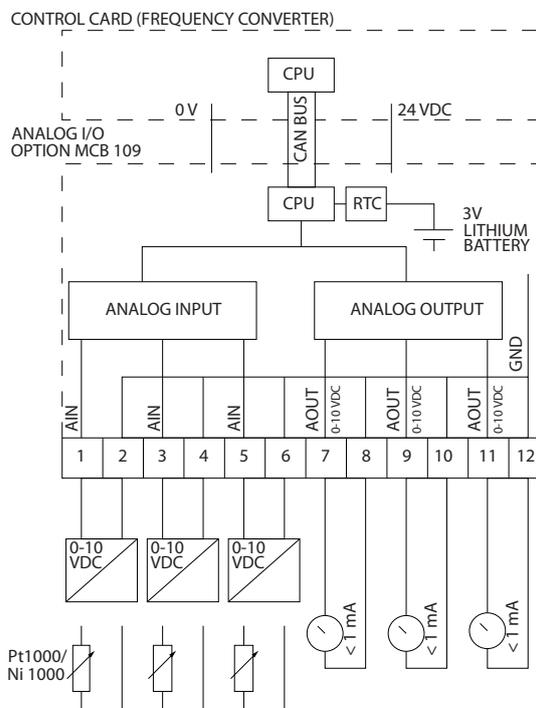
**Illustration 3.11 Principle Diagram for Analog I/O Mounted in the Frequency Converter**
