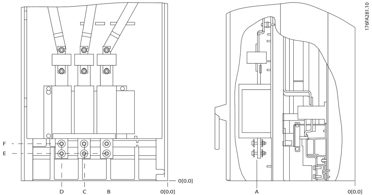
Illustration 5.81 IP00 Enclosure Power Connections, Position of Disconnect Switch
