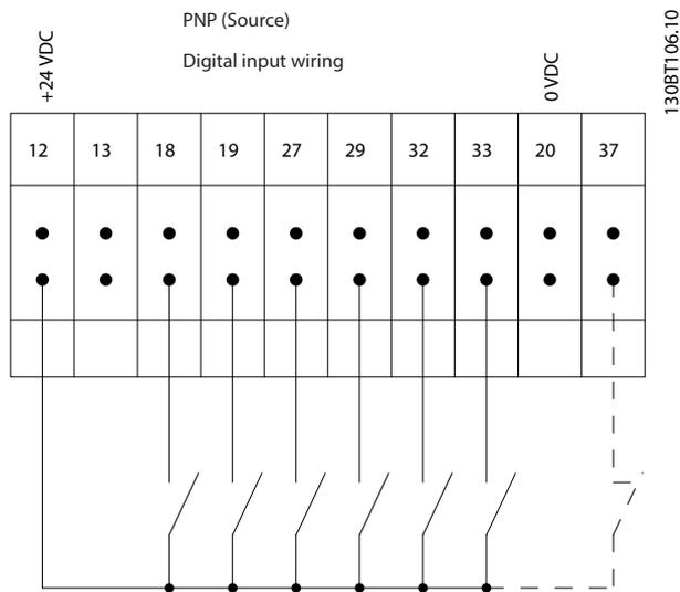
Illustration 5.57 Input Polarity of Control Terminals
