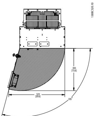
Illustration 5.12 Front Clearance of IP21/IP54 Enclosure Type, Frame Size D2h, D7h, and D8h.
