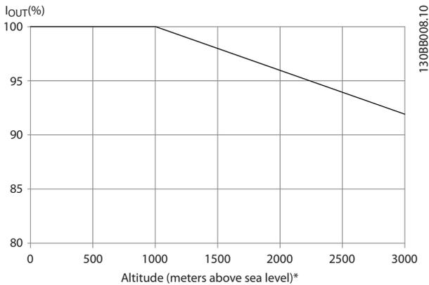
Illustration 3.3 Derating of Output Current Versus Altitude at  $T_{AMB, MAX}$
