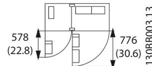
Illustration 5.14 Front Clearance of IP21/IP54 Enclosure Type, Frame Size F1
