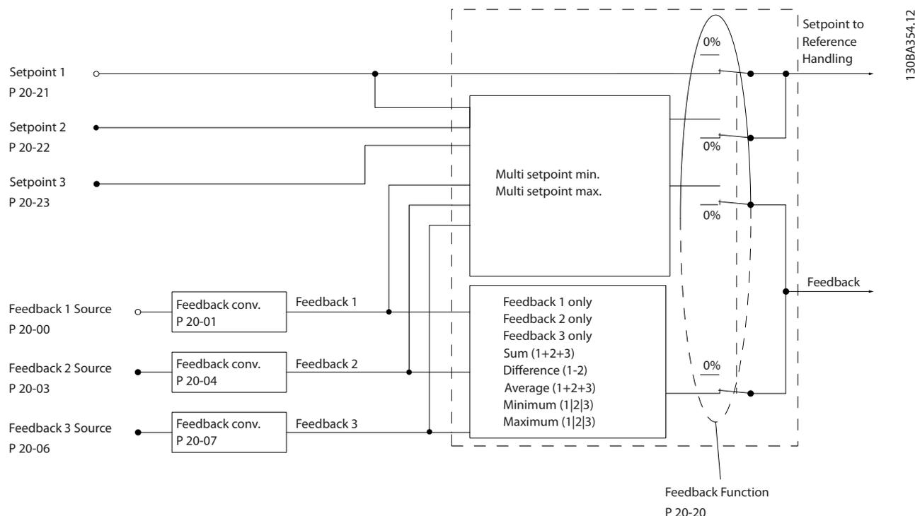
Illustration 2.13 Block Diagram of Feedback Signal Processing
