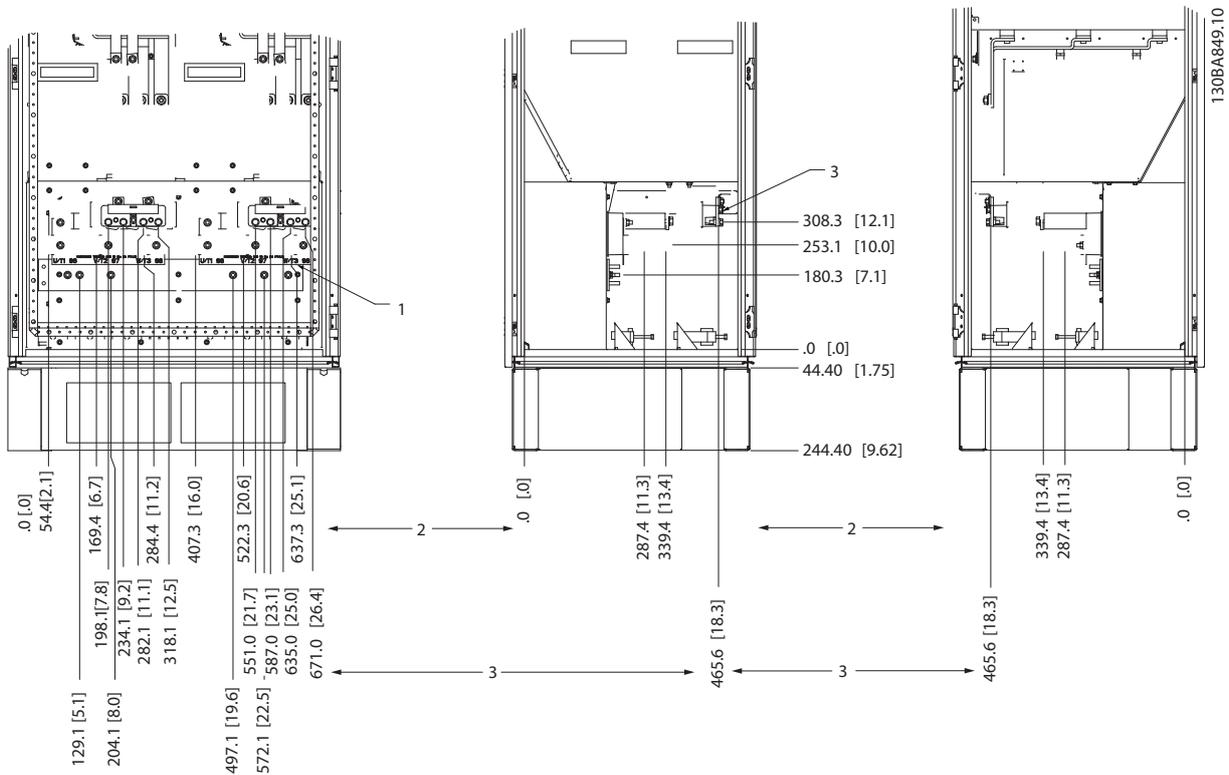
Illustration 5.83 Terminal Locations - Inverter Cabinet - F1 and F3 (Front, Left and Right Side View). The Gland Plate is 42 mm below .0 level.
