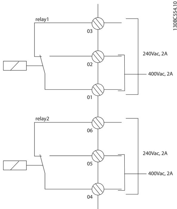
Illustration 5.100 D-frame Additional Relay Outputs
