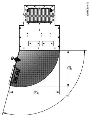
Illustration 5.11 Front Clearance of IP21/IP54 Enclosure Type, Frame Size D1h, D5h, and D6h.
