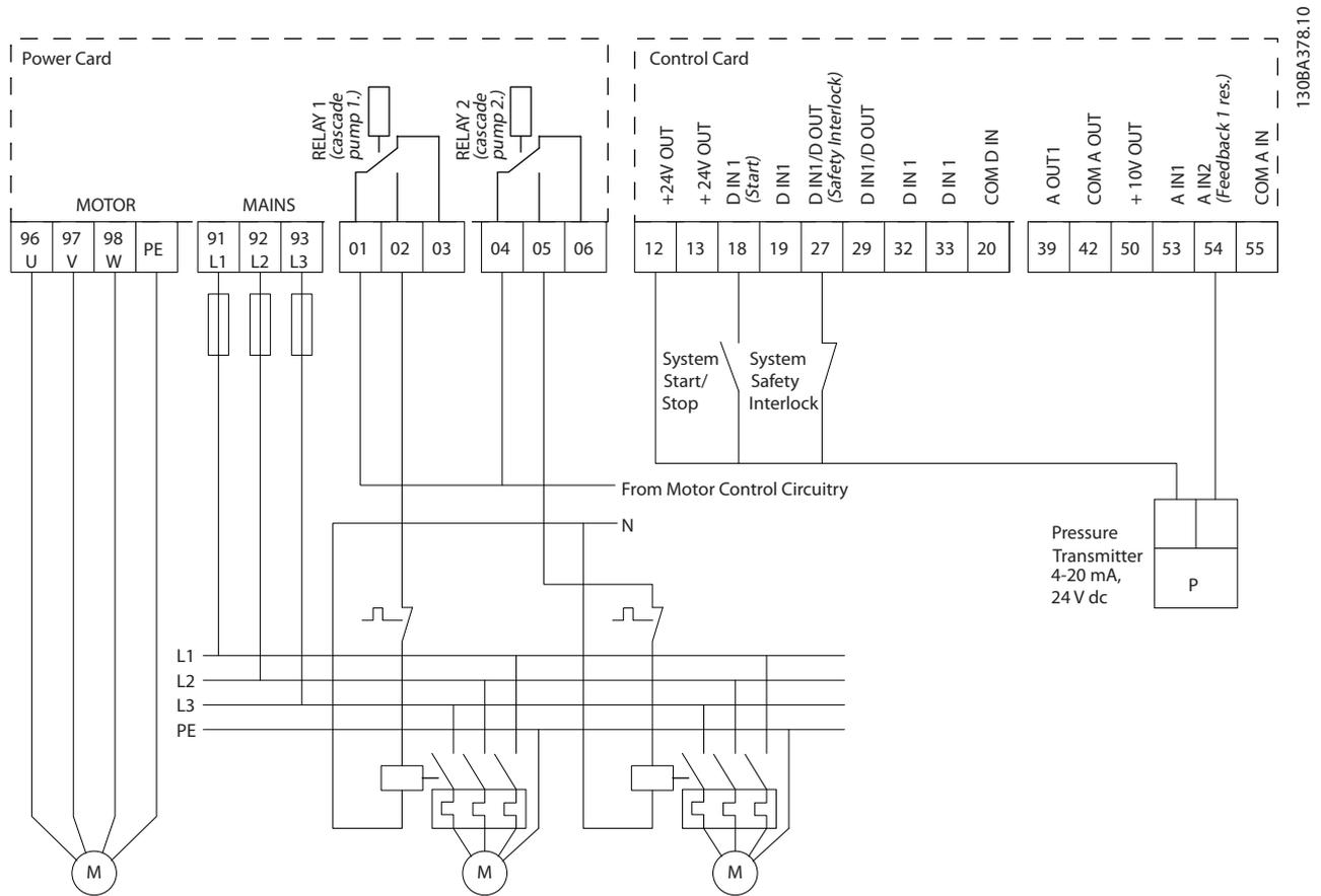
Illustration 6.9 Cascade Controller Wiring Diagram
