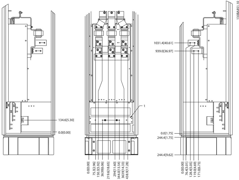
Illustration 5.88 Terminal Locations - Options Cabinet (Left, Front and Right Side View). The Gland Plate is 42 mm below .0 level.
