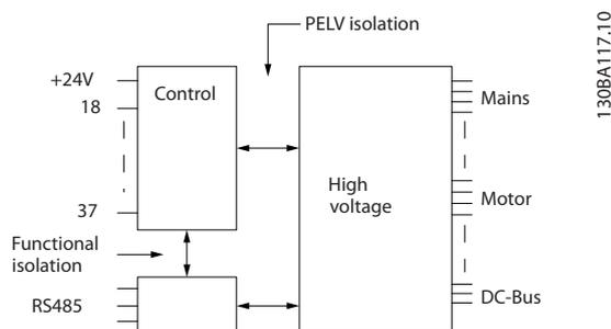
**Illustration 3.1 PELV Isolation of Analog Inputs**
