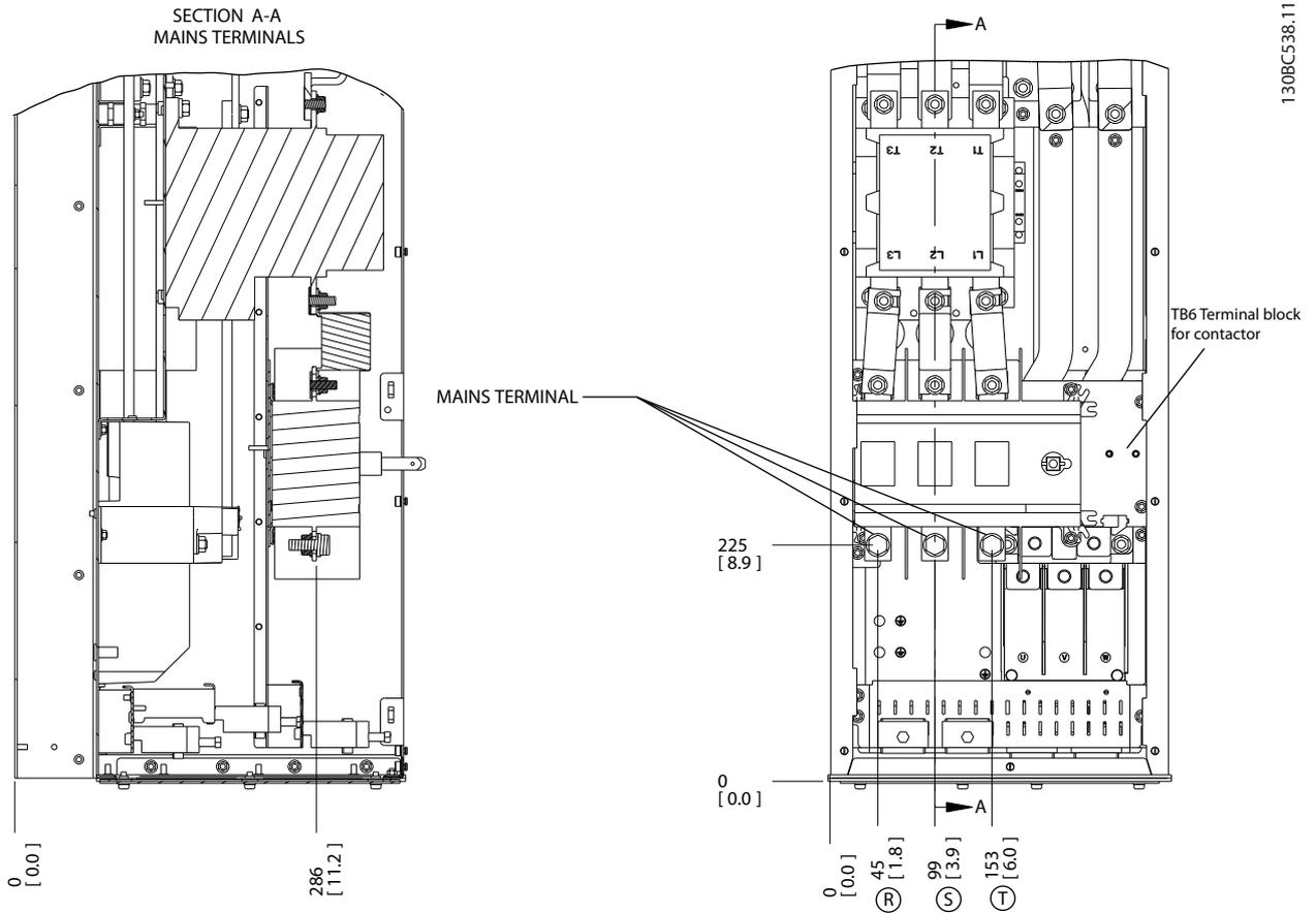
Illustration 5.69 Terminal Locations, D6h with Contactor and Disconnect Options
