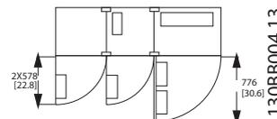
Illustration 5.15 Front Clearance of IP21/IP54 Enclosure Type, Frame Size F3
