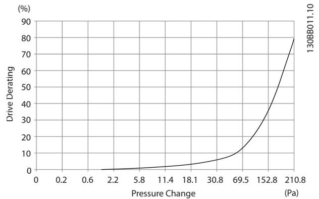
**Illustration 5.26 E-Frame Derating vs. Pressure Change (Large Fan), P315T5-P400T5 and P500T7-P560T7**
