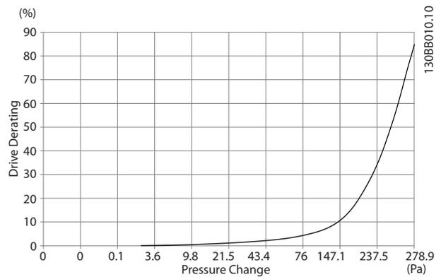
**Illustration 5.25 E-Frame Derating vs. Pressure Change (Small Fan), P250T5 and P355T7-P400T7**
