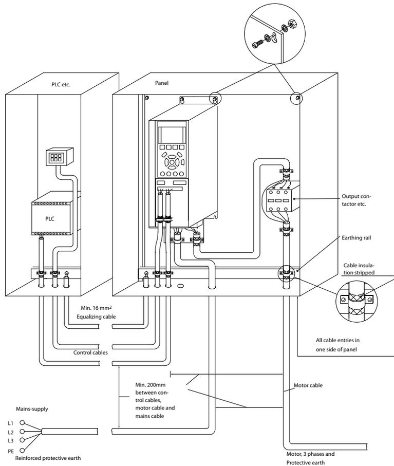
Illustration 5.106 EMC-correct Electrical Installation of a Frequency Converter in Cabinet
