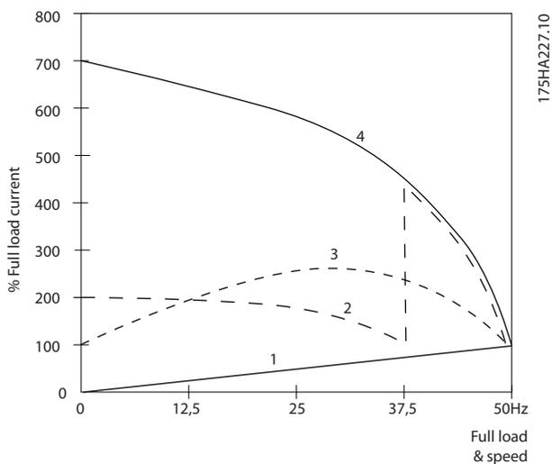
Illustration 2.6 Current Consumption with a Frequency Converter
