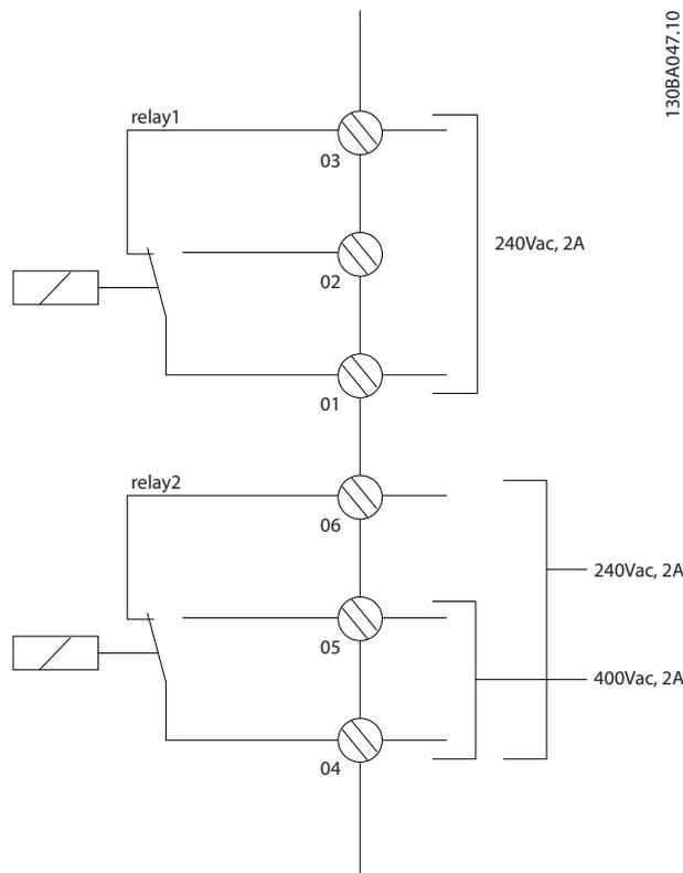
Illustration 5.101 E- and F-frame Additional Relay Outputs
