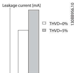
Illustration 2.22 Influence of Line Distortion on Leakage Current
