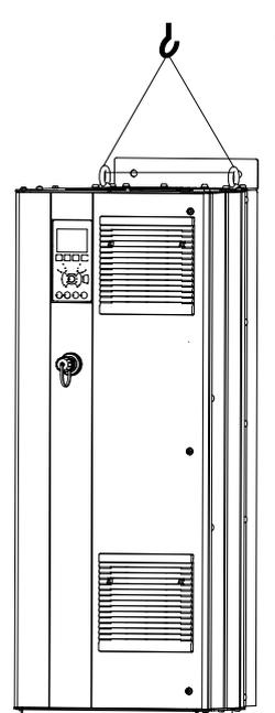
Illustration 5.6 Recommended Lifting Method, D-Frame Size
