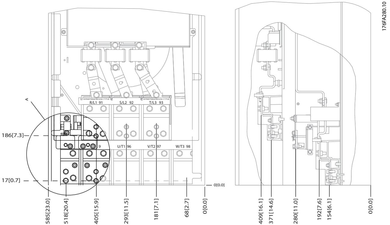
Illustration 5.79 IP00 Enclosure Power Connection Positions
