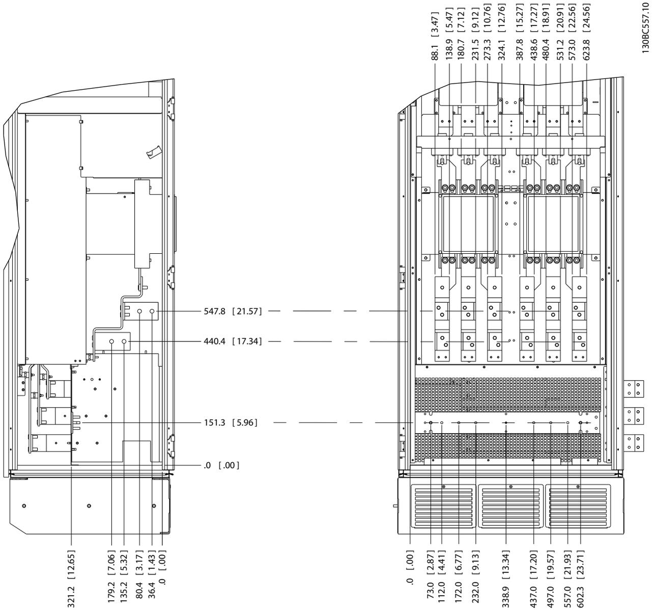
Illustration 5.97 F11/F13 Input Option Cabinet with Disconnect and Fuses
