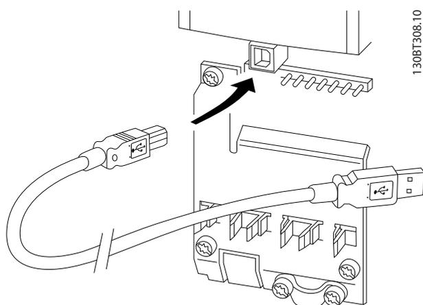
Illustration 5.105 Connection of PC to Frequency Converter
