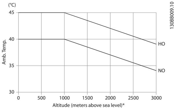
Illustration 3.4 Derating of Output Current Versus Altitude at  $T_{AMB, MAX}$
