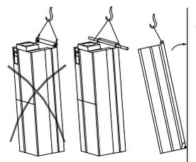
Illustration 5.7 Recommended Lifting Method, E-Frame Size
