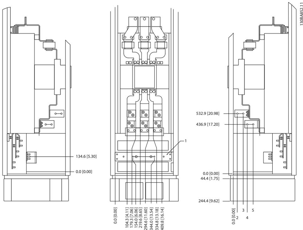
Illustration 5.89 Terminal Locations - Options Cabinet with Circuit Breaker/Molded Case Switch (Left, Front and Right Side View). The Gland Plate is 42 mm below .0 level.
