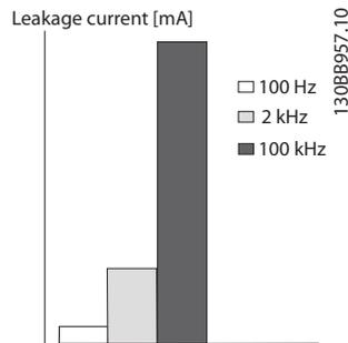
Illustration 2.24 The Influence of the Cut-off Frequency of the RCD on what is responded to/measured
