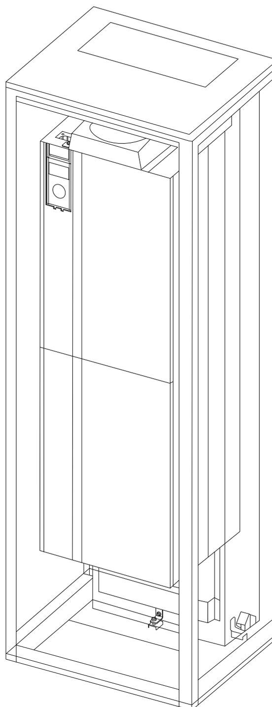
Illustration 3.19 Installation of IP00/IP20/Chassis in Rittal TS8 Enclosure.
