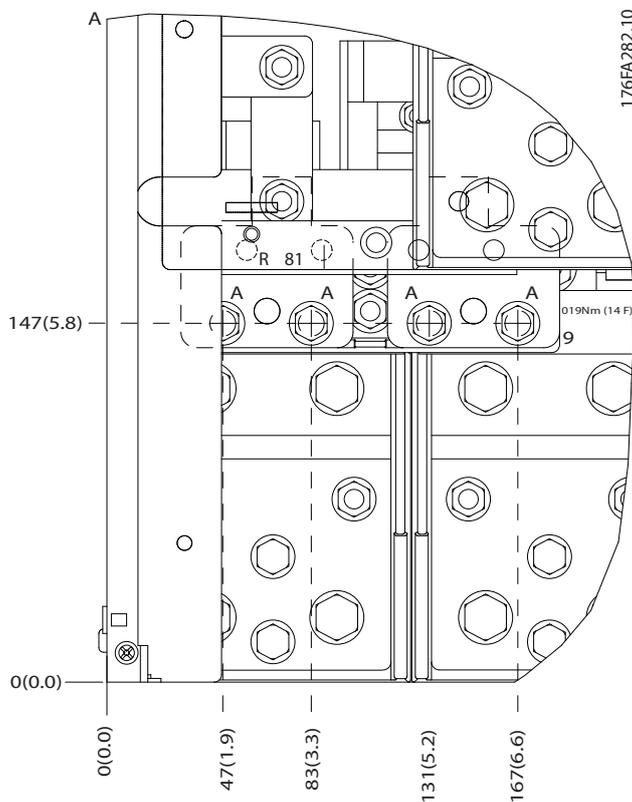
Illustration 5.80 IP00 Enclosure Power Connection Positions
