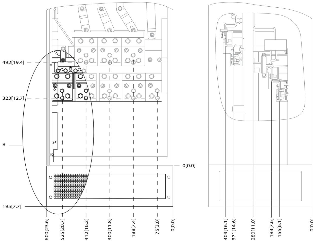
**Illustration 5.76 IP21 (NEMA Type 1) and IP54 (NEMA Type 12) Enclosure Power Connection Positions**
