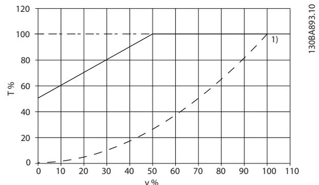
Illustration 3.5 Maximum Load for a Standard Motor at 40 °C
