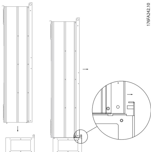
**Illustration 3.22 Mounting of the Frequency Converter to the Pedestal**
