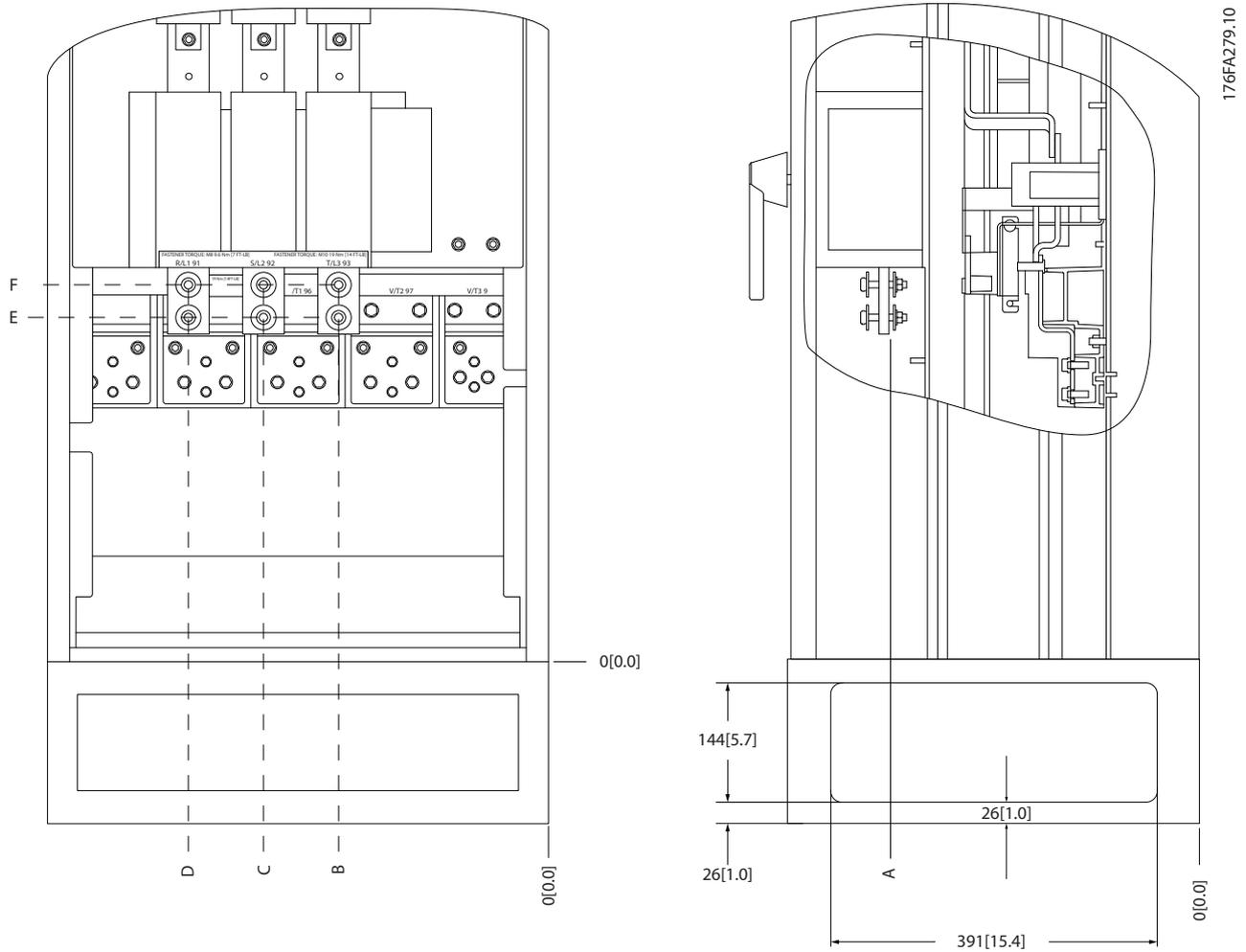
Illustration 5.78 IP21 (NEMA type 1) and IP54 (NEMA type 12) Enclosure Power Connection Position of Disconnect Switch
