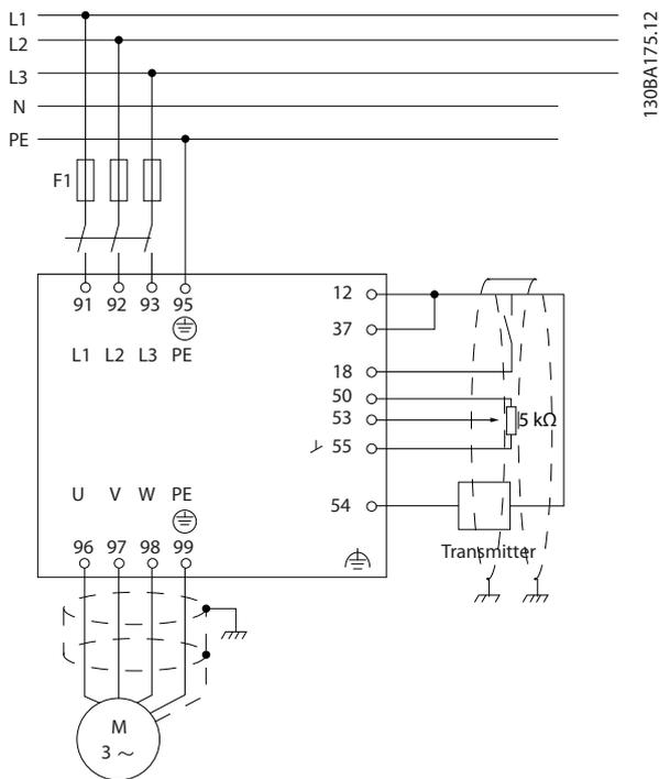
Illustration 5.107 Electrical Connection Diagram (6-pulse example shown)
