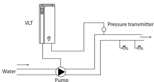
Illustration 2.16 Closed Loop PID Control
