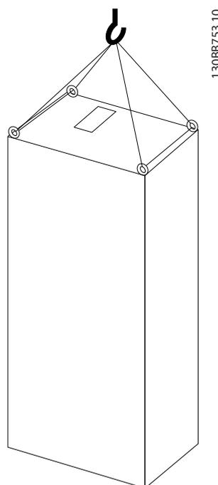
Illustration 5.10 Recommended Lifting Method, Frame Sizes F8
