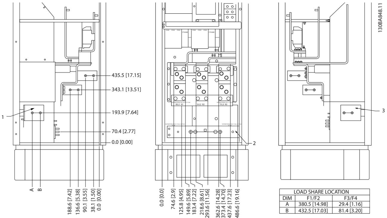
Illustration 5.87 Terminal Locations - Rectifier (Left, Front and Right Side View). The Gland Plate is 42 mm below .0 level.
