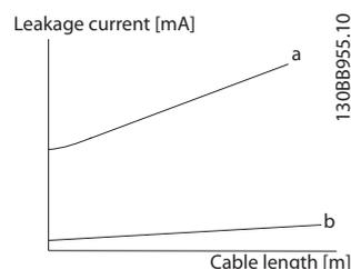
Illustration 2.21 Influence of the Cable Length and Power Size on the Leakage Current.  $P_a > P_b$
