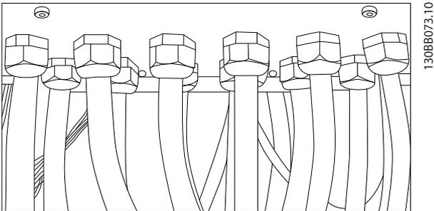
Illustration 5.28 Example of Proper Installation of Gland Plate
