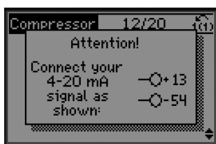
Illustration 3.13 Info: 4-20 mA Feedback Chosen - Connect Accordingly
