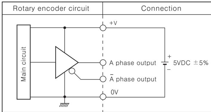
※All output circuit is the same A,  $\bar{A}$ , B,  $\bar{B}$ , Z,  $\bar{Z}$  phase.
